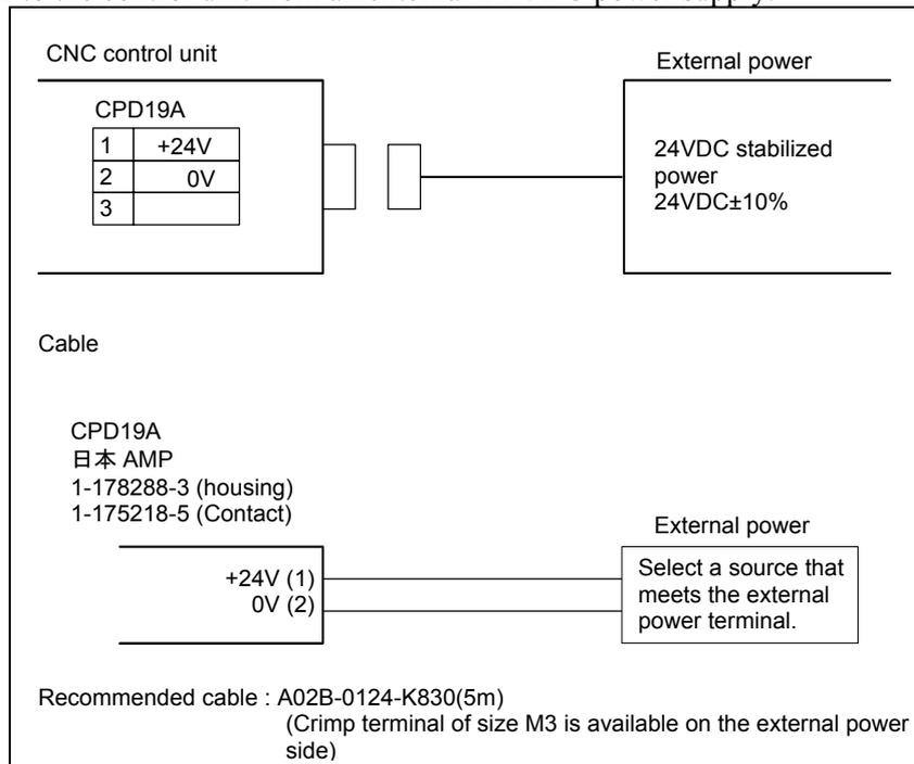
As for an stand-alone type control unit, part of the 24 VDC power input to CPD19A can be taken out from CPD19B by branching. CPD19B should be connected as shown below. In this case, the rating of the external 24 VDC power supplied to CPD19A must be the sum of the power consumed within the control unit and that supplied to external equipment via CPD19B. Up to 1.0 A can be supplied to the external equipment.
