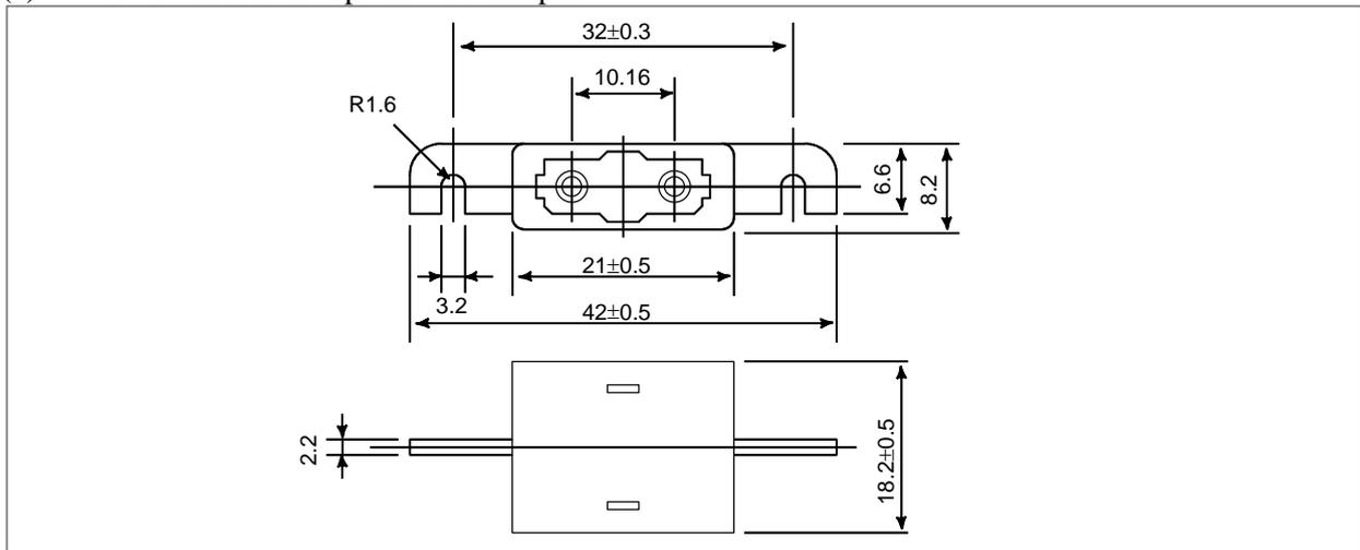
(b) Example of the use of an optical fiber adapter
