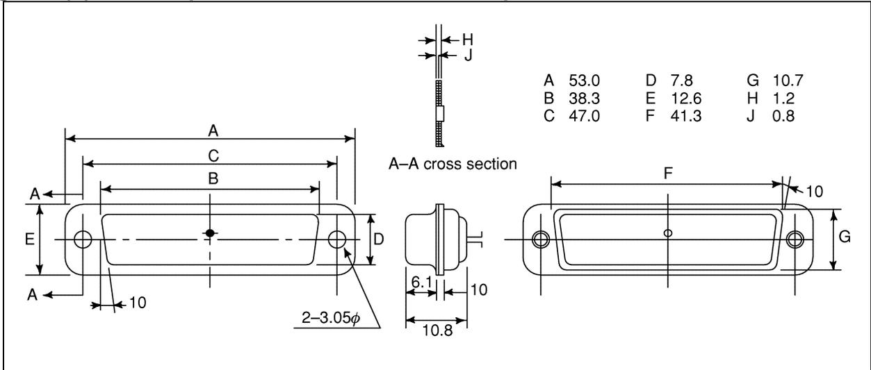
**Fig. C8 (b) Locking plate plate for reader/puncher interface connector**
