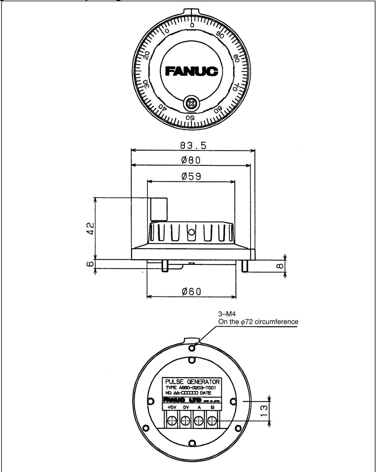
**Fig. U19 Pendant type manual pulse generator**
