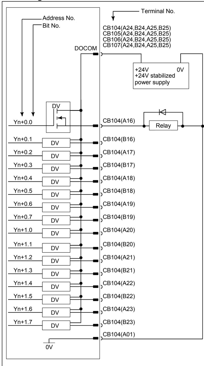
9.CONNECTION OF I/O Link SLAVE DEVICES
