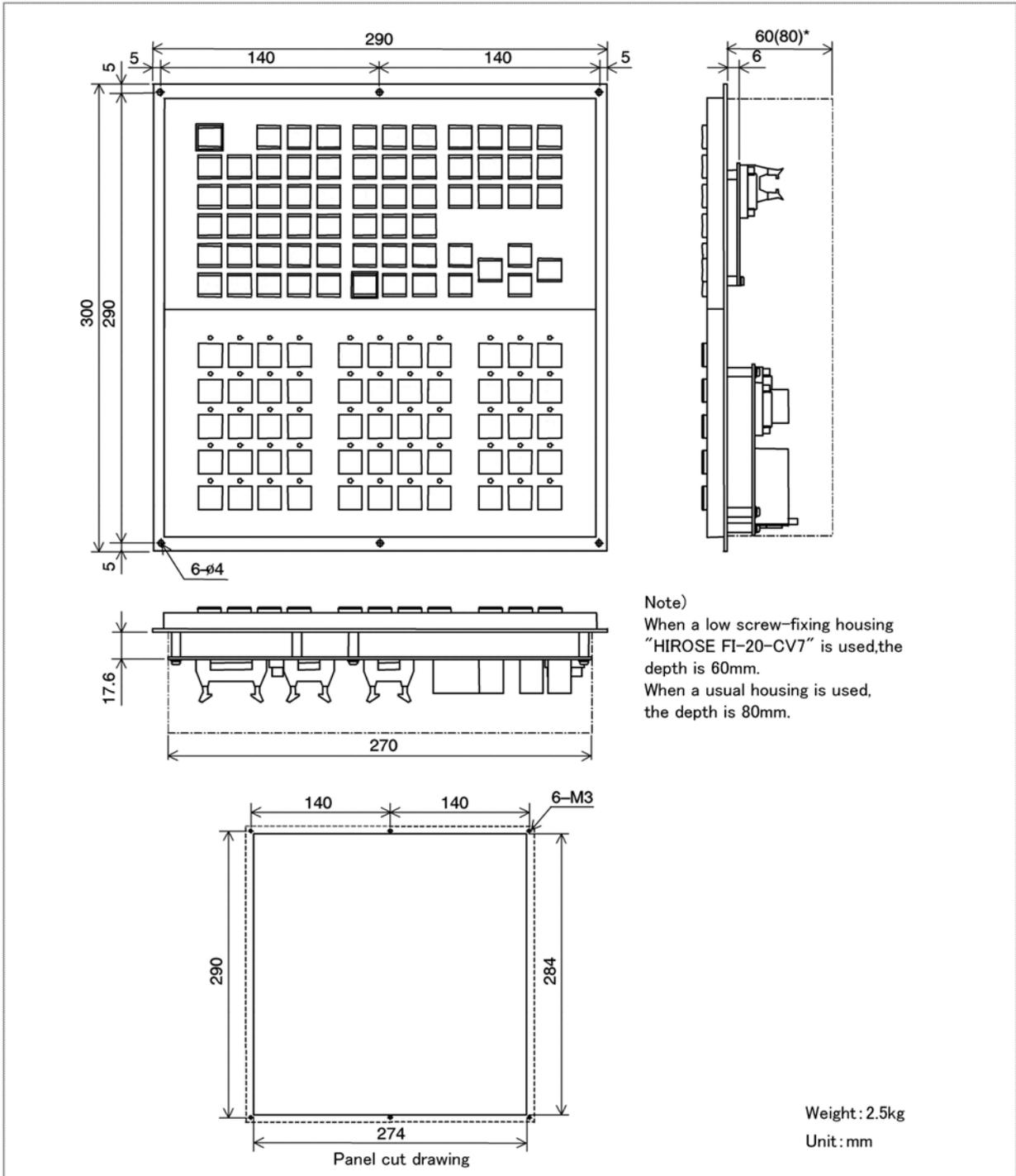
**Fig. U26 Machine operator's panel: Main panel B**
