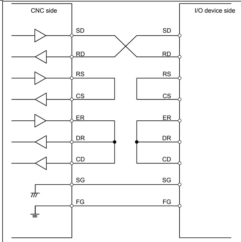
he cable for connecting the I/O device to the CNC should be connected as shown in the below diagram.
