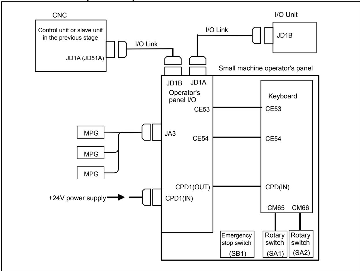
**For small machine operator's panel B**
