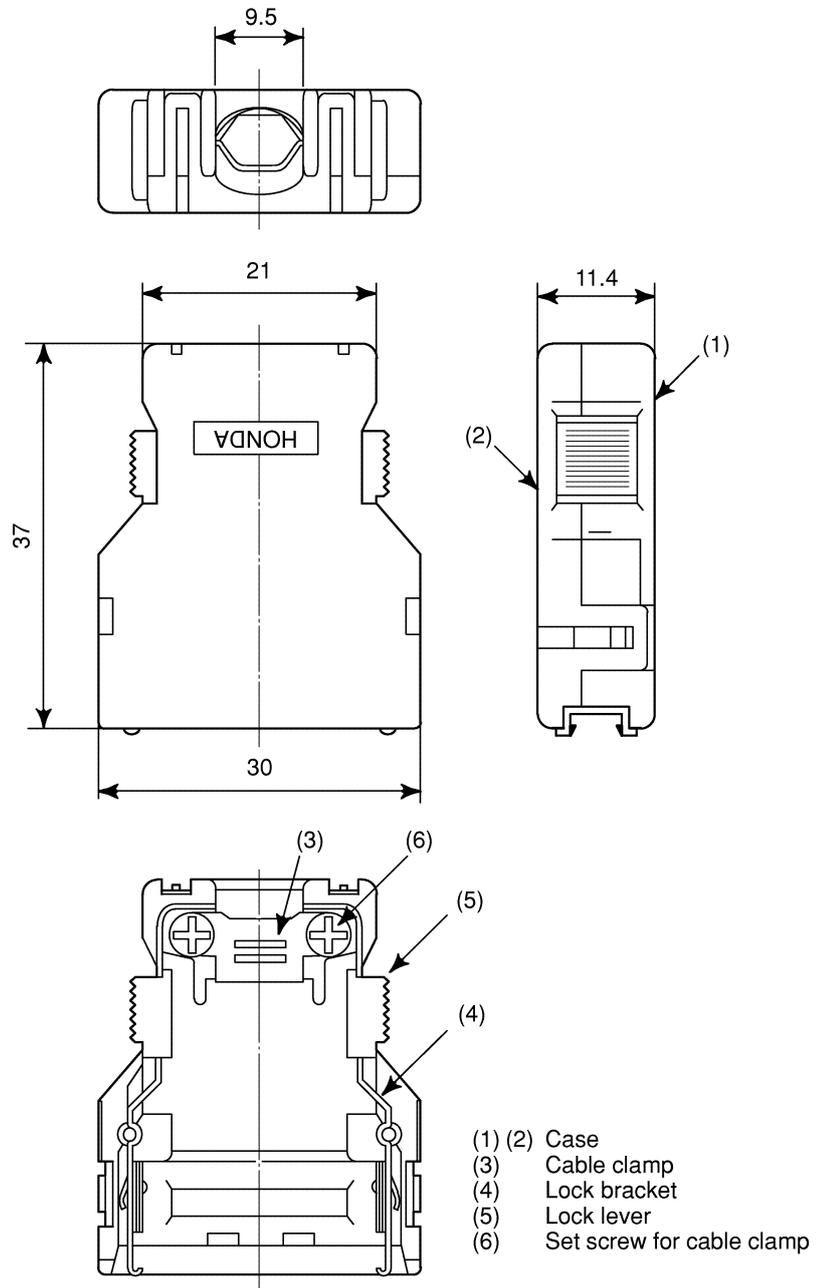
**Fig. C2 (b) Connector case (HIROSE FI type)**
