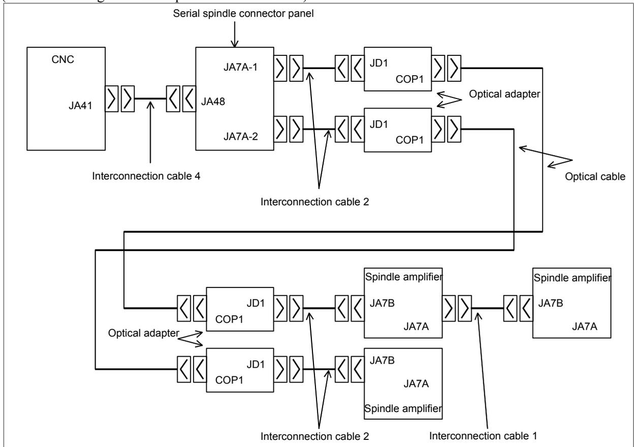
(Cable connections when only electrical cables are used)
