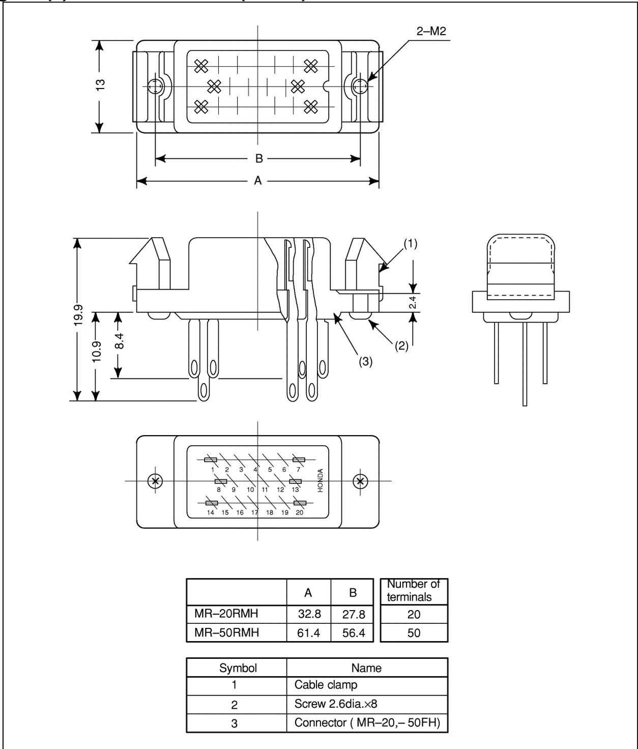
**Fig. C4 (e) HONDA connector (terminal layout)**
