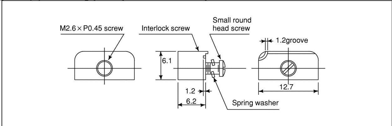
**Fig. C9 Honda connector (for the distributed I/O connector printed circuit board)**
