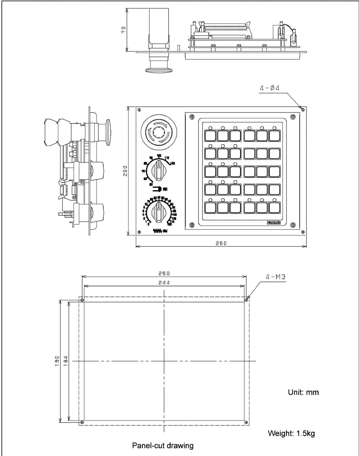
**9.10.8.2 Layout of the key sheet (Same for both the small machine operator's panel and small machine operator's panel B)**
