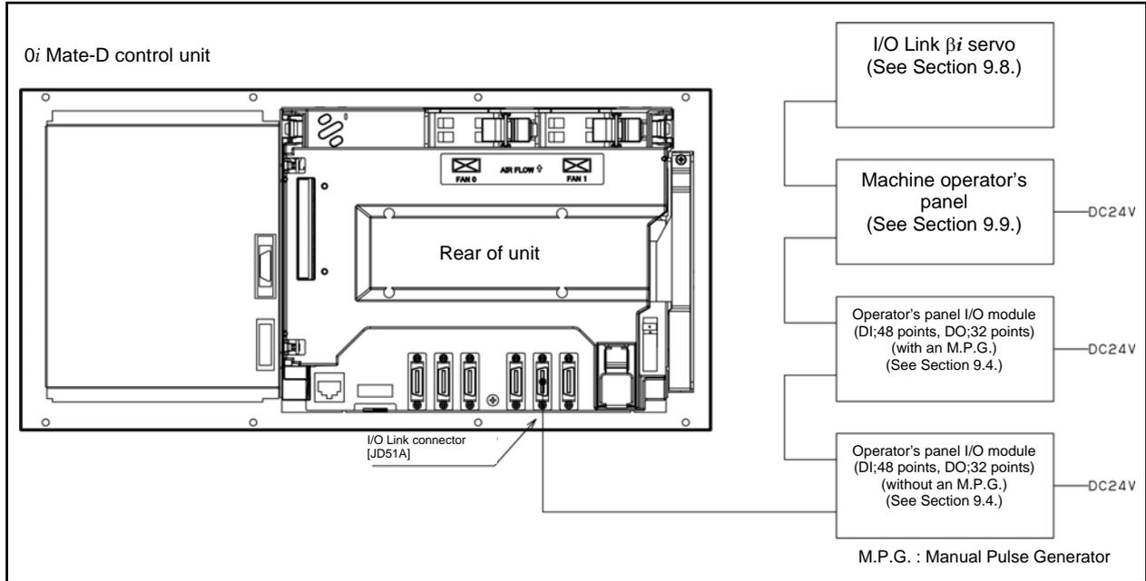
The following example assumes that two operator's panel I/Os and one machine operator's panel are used.
