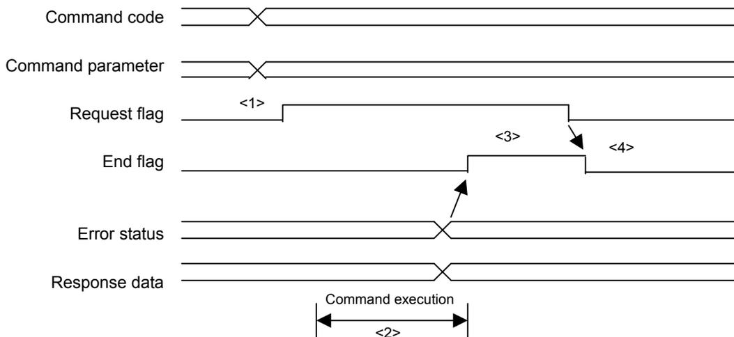
**<1> PMC side:** Command code is written after checking that both of the request flag and end flag are OFF. If the command has parameter data, the parameter data is written simultaneously. Next, the request flag is set to ON. Within the same scan period, command code may be written and the request flag may be set to ON.
