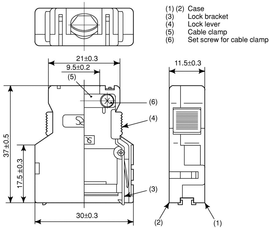
**Fig. C2 (c) Connector case (FUJITSU FCN type)**
