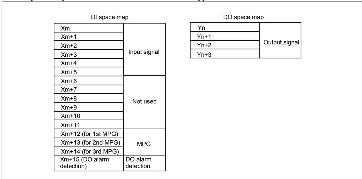
Basically, this 48/32-point I/O module is allocated a group of DI addresses (16 bytes) and a group of DO addresses (4 bytes). This address allocation is explained below.
