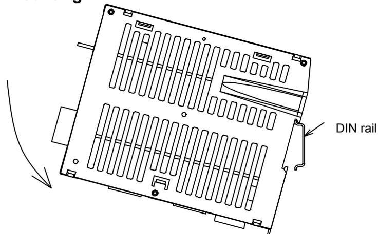
1. Place the hook of the unit onto the top of the DIN rail.
