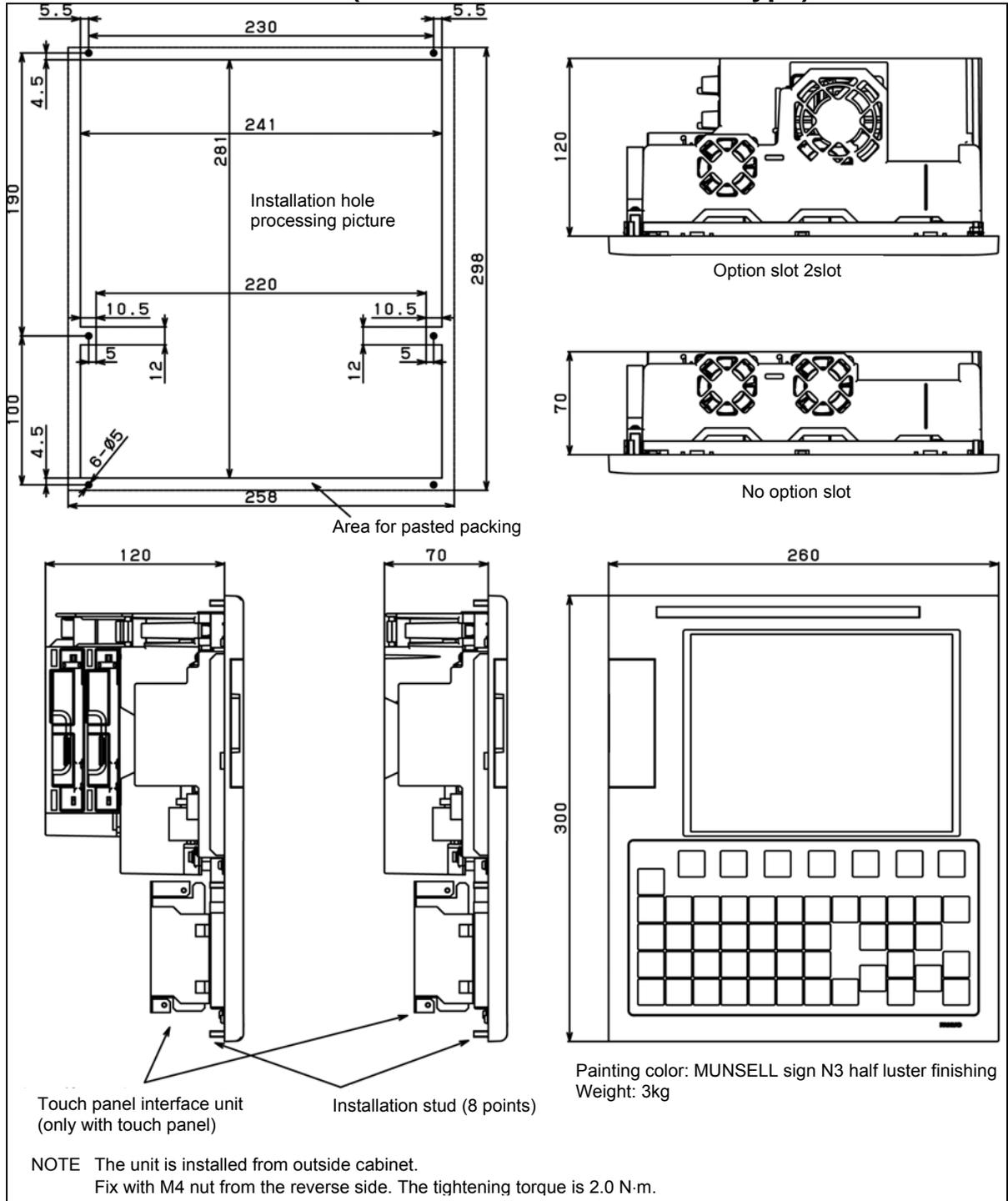
**Fig. U3 CNC control unit (10.4" color LCD)**
