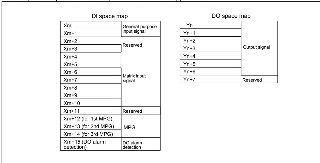
The operator's panel I/O module is allocated a group of DI addresses (16 bytes) and a group of DO addresses (8 bytes). This address allocation is explained below.
