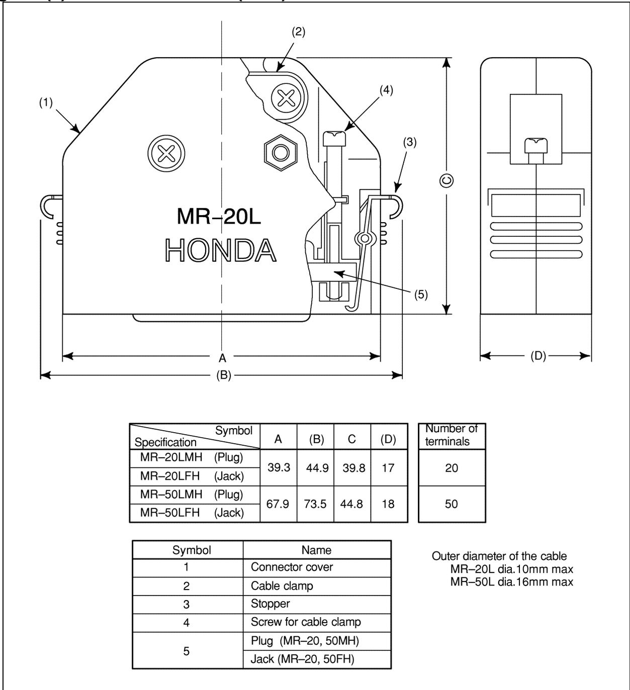
**Fig. C4 (b) Honda connector (angled-type case)**
