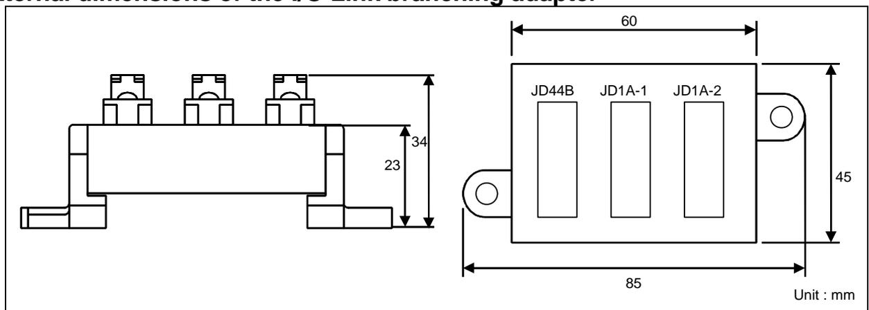
Allow a clearance of about 10 cm above the adapter for connection and routing of cables.
