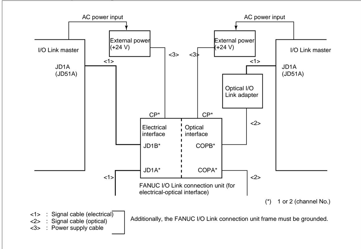
[Name of I/O Link connection unit connectors]
