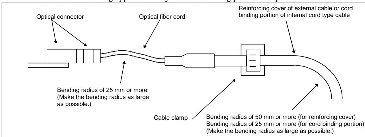
**Fig. D(e) Fixing the cable with a clamp**
