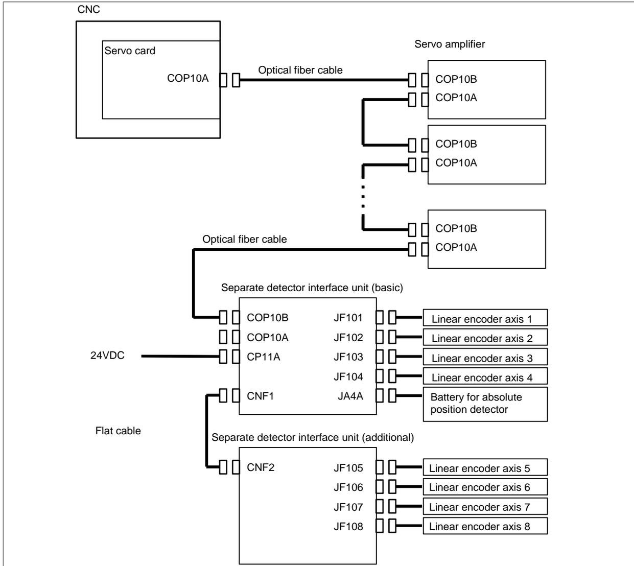
When a separate detector such as a separate rotary encoder or linear encoder is used, a separate detector interface unit is required. The separate detector interface unit is connected through an optical fiber cable as an unit on an FSSB line.
