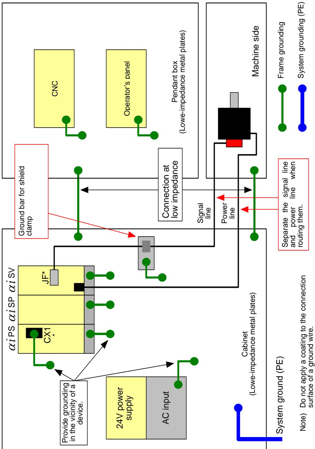
Fig. 3.5.1.2 (a) Schematic diagram for multipoint grounding scheme
