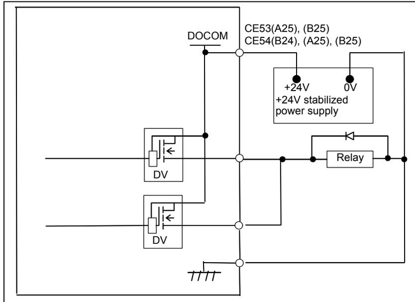
**DO (output signal) alarm detection**
