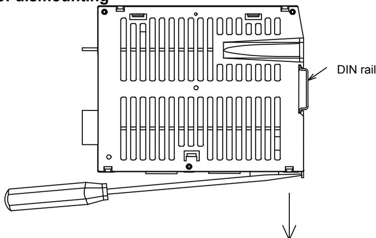
1. Lower the locking section with a flat-blade screwdriver.
