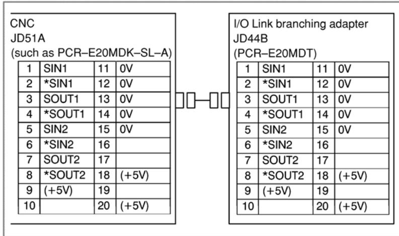
The +5V pin is provided to use the optical I/O Link adapter for optical fiber transmission. When not using the optical I/O Link adapter, leave the +5V pin unconnected.
