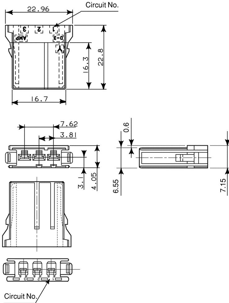
**Fig. C3 (e) Contact for AMP connector**
