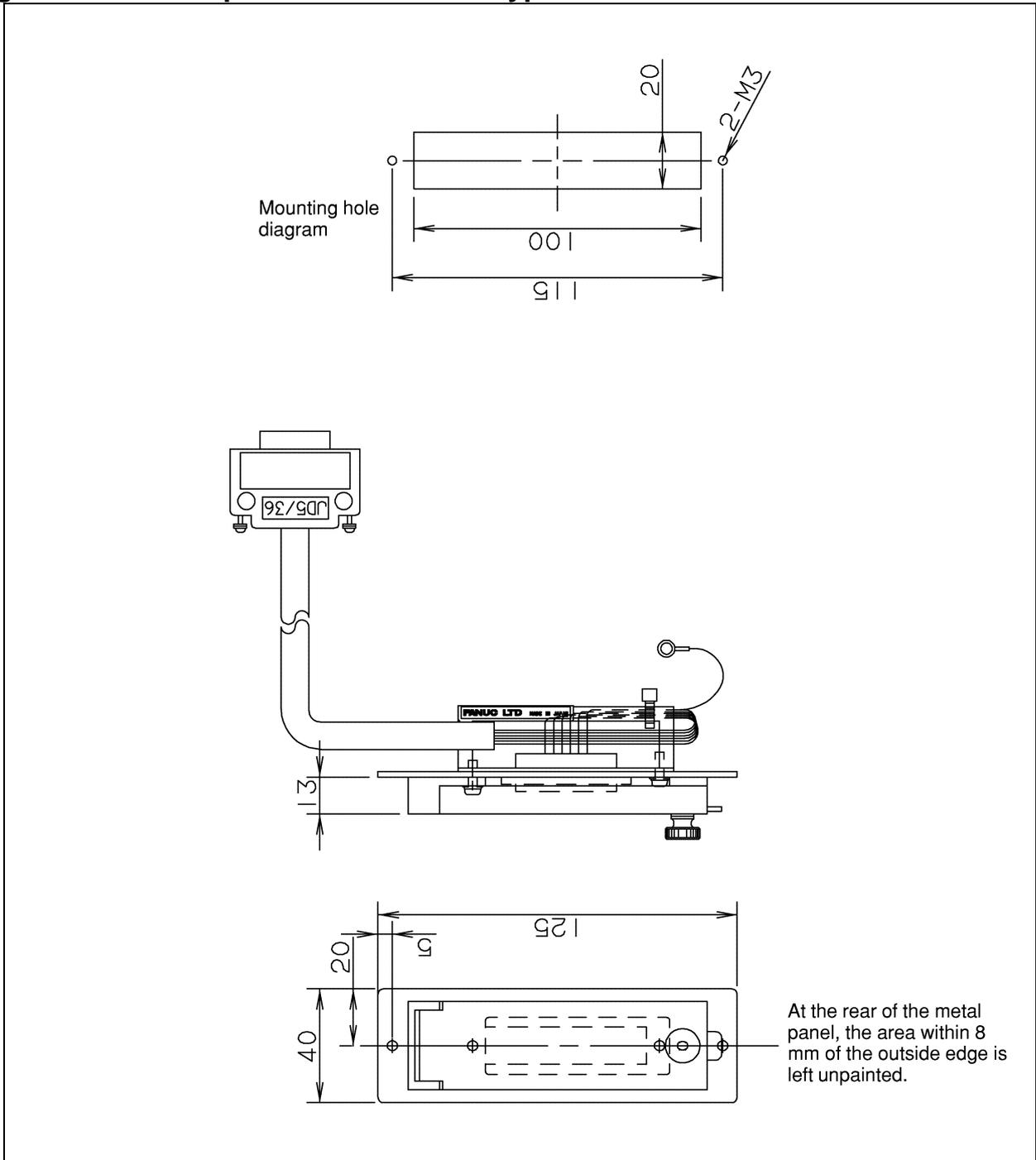
**Fig. U25 Machine operator's panel: Main panel A**
