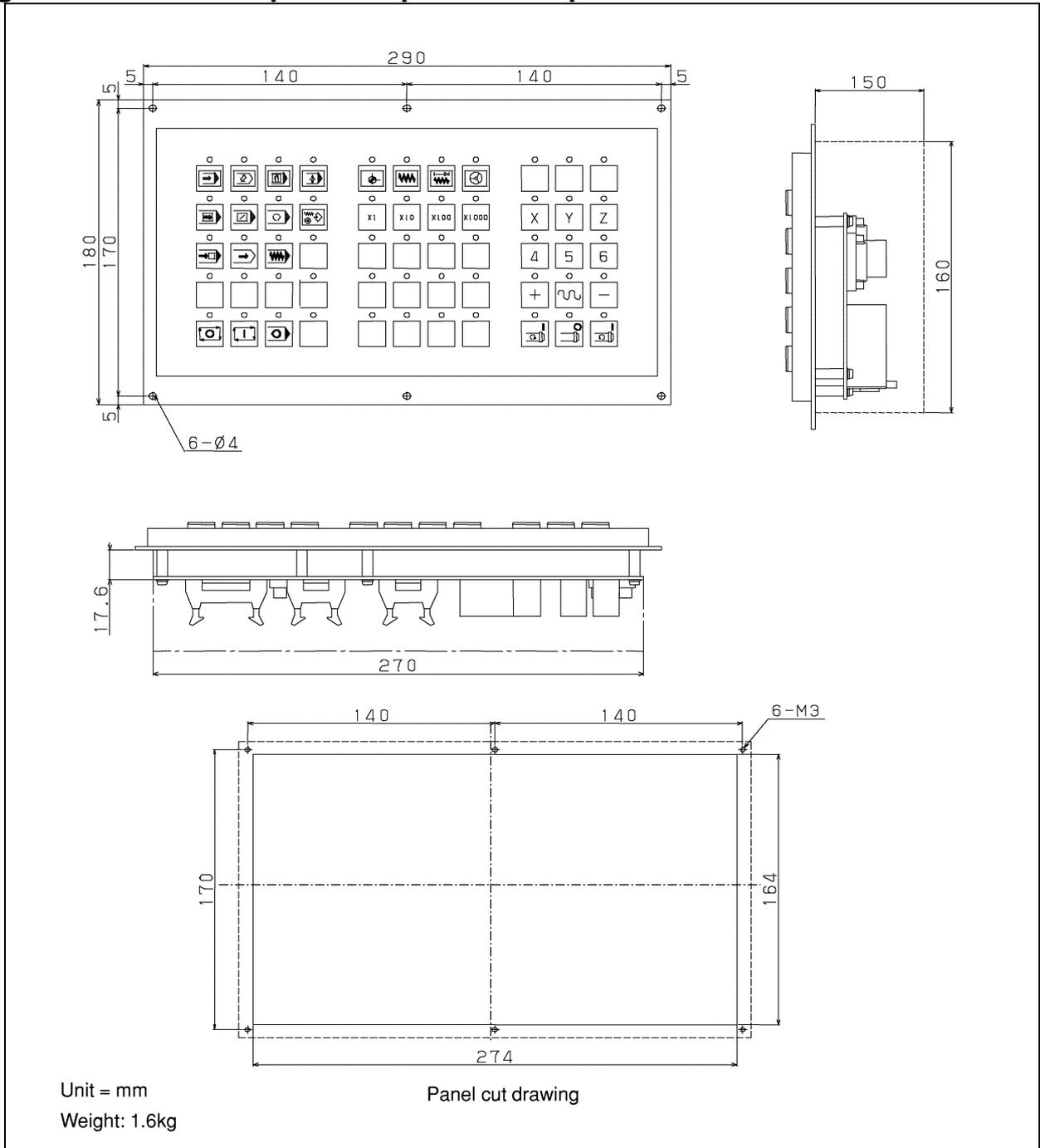
**Fig. U27 Machine operator's panel: Sub panel A**
