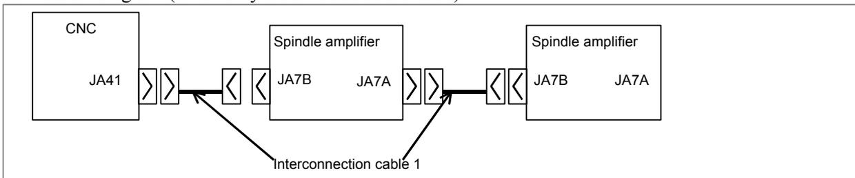
Connection diagram (when an optical cable is used)
