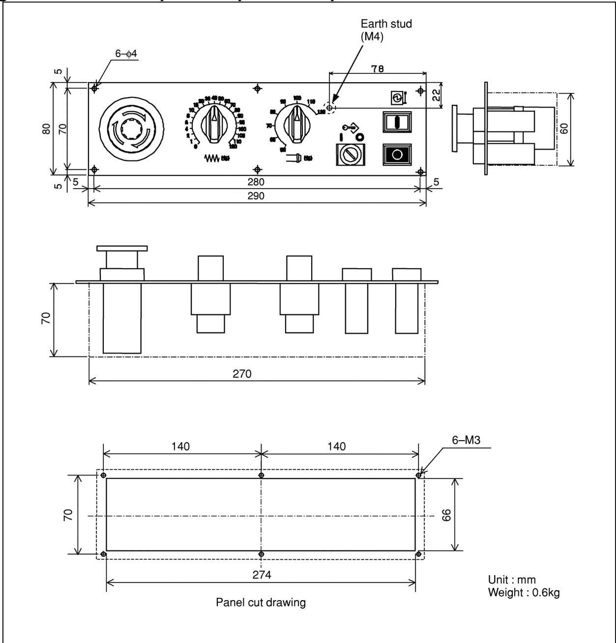
**Fig. U28 Machine operator's panel: Sub panel B1**
