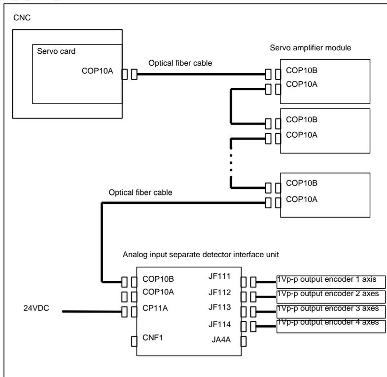
(2) Connecting 1-Vp-p output encoders to the 5th to 8th axes
