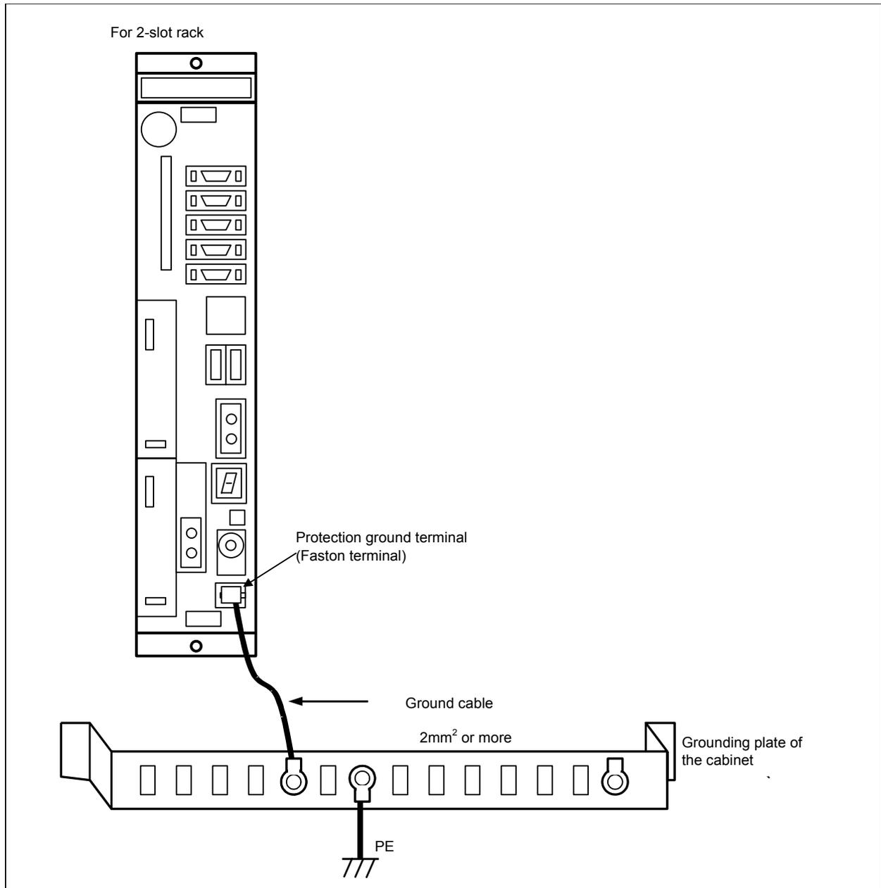
Connect the 0-V lines of the electronic circuits in the control unit to the ground plate of the cabinet via the protection ground terminal (above figure).
