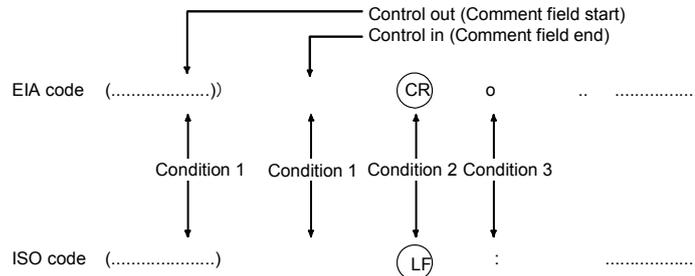
**Condition1** Left parenthesis "(" of the ISO code punches holes at bits 2, 4 and 5 when used in the EIA code.
