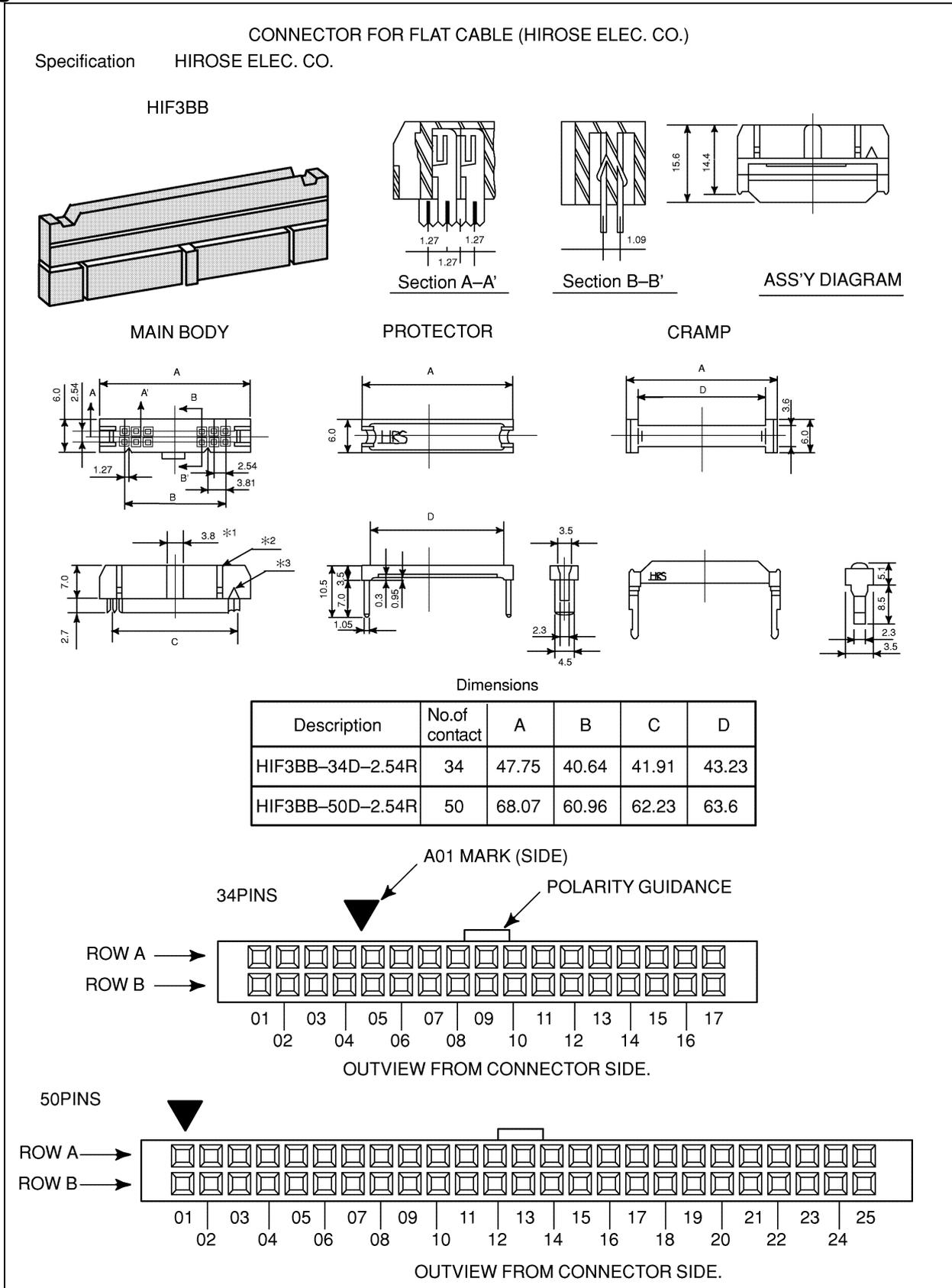
**Fig. C8 (a) Punch panel connector for reader/puncher interface**
