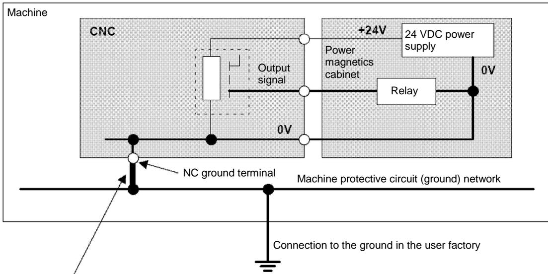
This bold line indicates grounding for the control unit described in the connection manual. As shown in this figure, by just connecting the ground terminal of the control unit to the machine ground, the 0 V output of the relay circuit in the power magnetism cabinet is connected to the ground (protective circuit).
