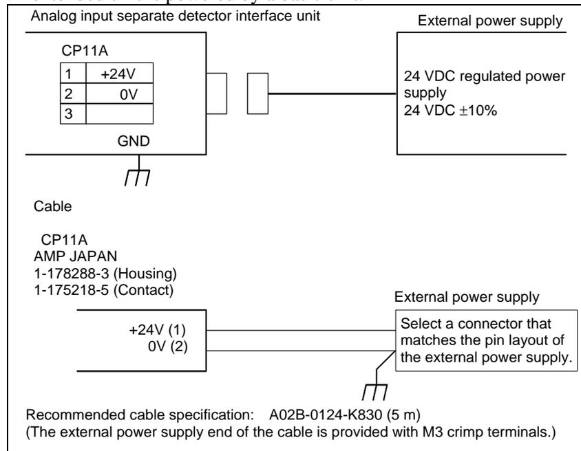
The 24 VDC input to CP11A can be output at CP11B for use in branching. The connection of CP11B is identical to that of CP11A. In this case, the power supplied to CP11A should be equal to the sum of the rating of the analog input separate detector interface unit and that of the units after CP11B.
