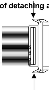
When detaching a connected cable from a module, release the lock by pushing the latch of the connector on the cable side in the arrow directions shown at the left.
