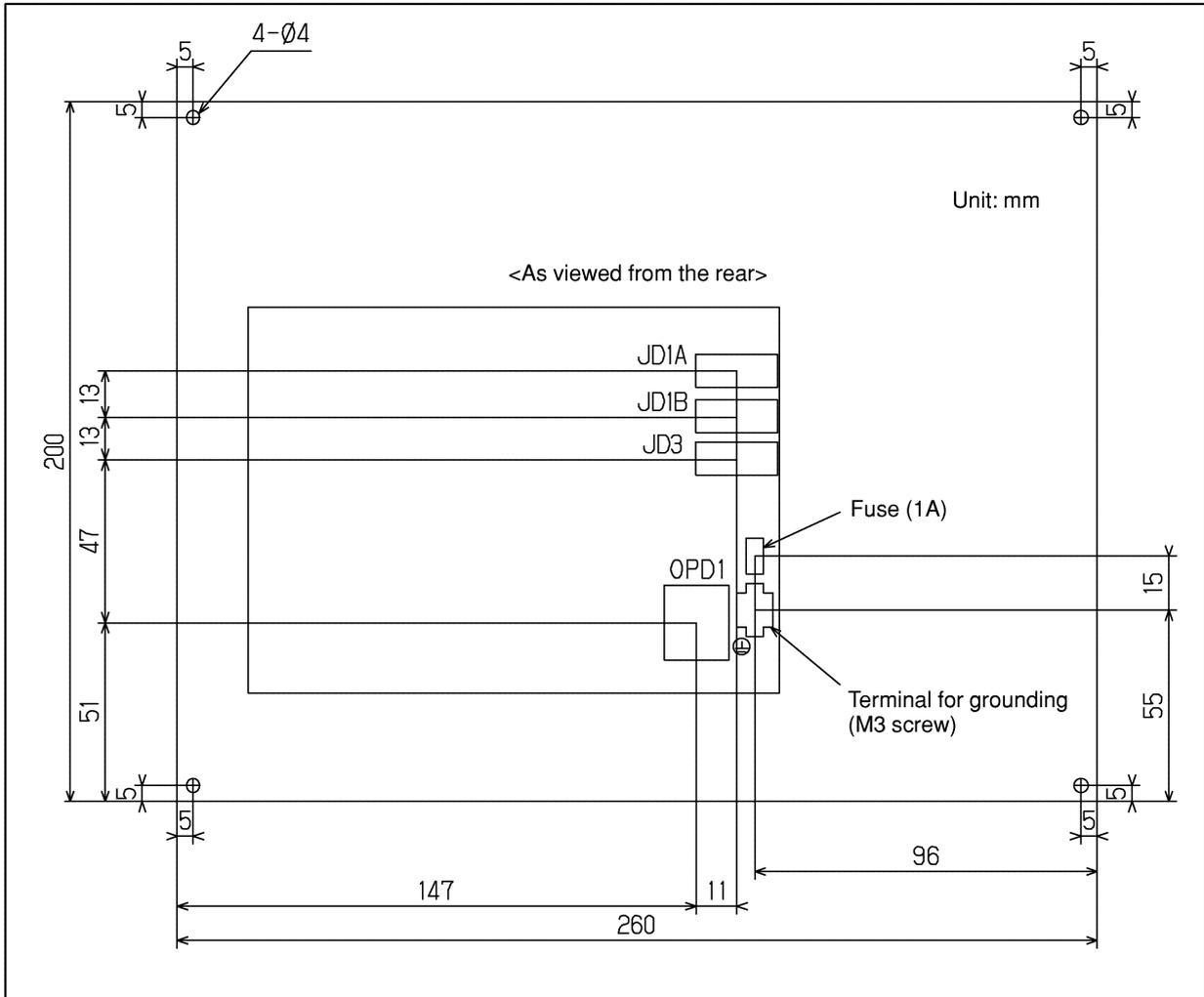
**Connector Layout of the small machine operator's panel B**
