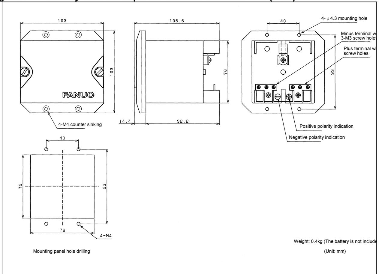
**Fig. U22 CNC battery unit for external installation**
