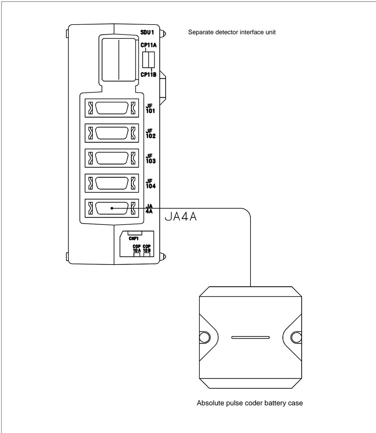
When the separate absolute position detector that needs battery backup is connected, the battery case for the separate absolute pulse coder must be connected.
