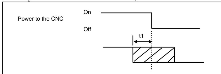
$t_1:500\text{ms}$  Means that the power to units are turned off within 500 ms before the power to the CNC is turned off.
