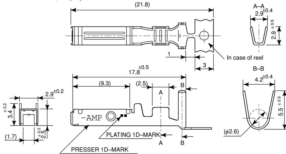
**Fig. C4 (a) HONDA connector (case)**
