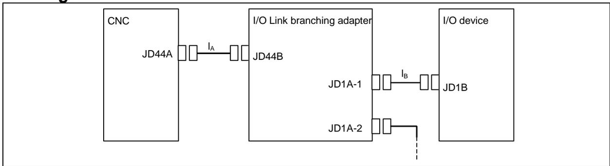
The total of  $l_A$  and  $l_B$  must not exceed 10 m; where  $l_A$  is the length of the cable between connector JD44A on the CNC and connector JD44B on the I/O Link branching adapter, and  $l_B$  is the length of the cable between connector JD1A-1 or JD1A-2 on the I/O Link branching adapter and connector JD1B on the I/O unit. When all cables are accommodated in the same cabinet, however, a total cable length of up to 15 m is allowed.
