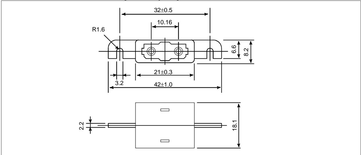
(b) Example of use of the optical fiber relay adapter
