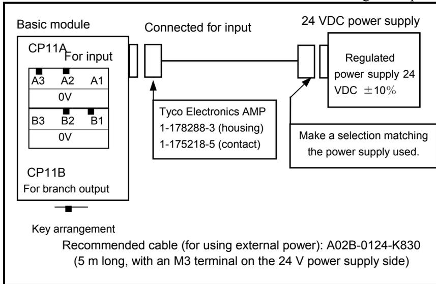
The 24 VDC input to CP11A (A1, A2) can be output from CP11B (B1, B2) for branching. CP11B (B1, B2) is connected as shown below. In this case, the external 24 VDC power supply needs to provide CP11A (A1, A2) with a current which is equal to the sum of the current consumed by the control unit and the current used via CP11B (B1, B2).
