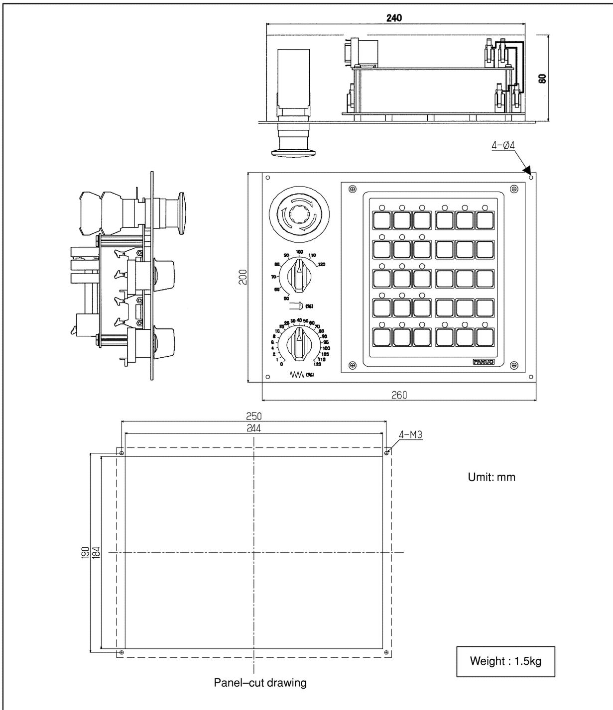
**Small machine operator's panel B**
