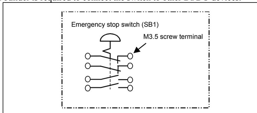
With the small machine operator's panel B, the input (pin 02) of the emergency stop input connector (CE74) is connected to general-purpose DI address Xm2+4.4 in the I/O board as shown below.
