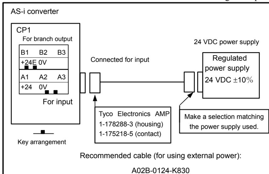
The 24 VDC input to CP1 (A1, A2) can be output from CP1 (B1, B2) for branching. CP1 (B1, B2) is connected as shown below. In this case, the external 24 VDC power supply needs to provide CP1 (A1, A2) with a current which is equal to the sum of the current consumed by the control unit and the current used via CP1 (B1, B2).
