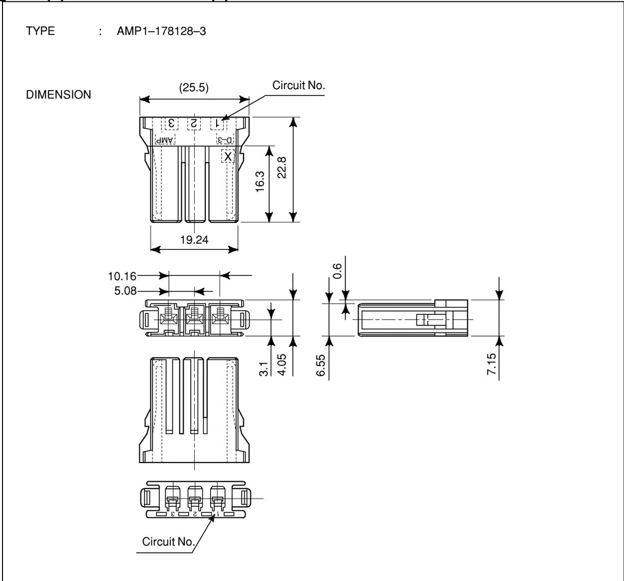
**Fig. C3 (b) AMP connector (2): On the servo side**
