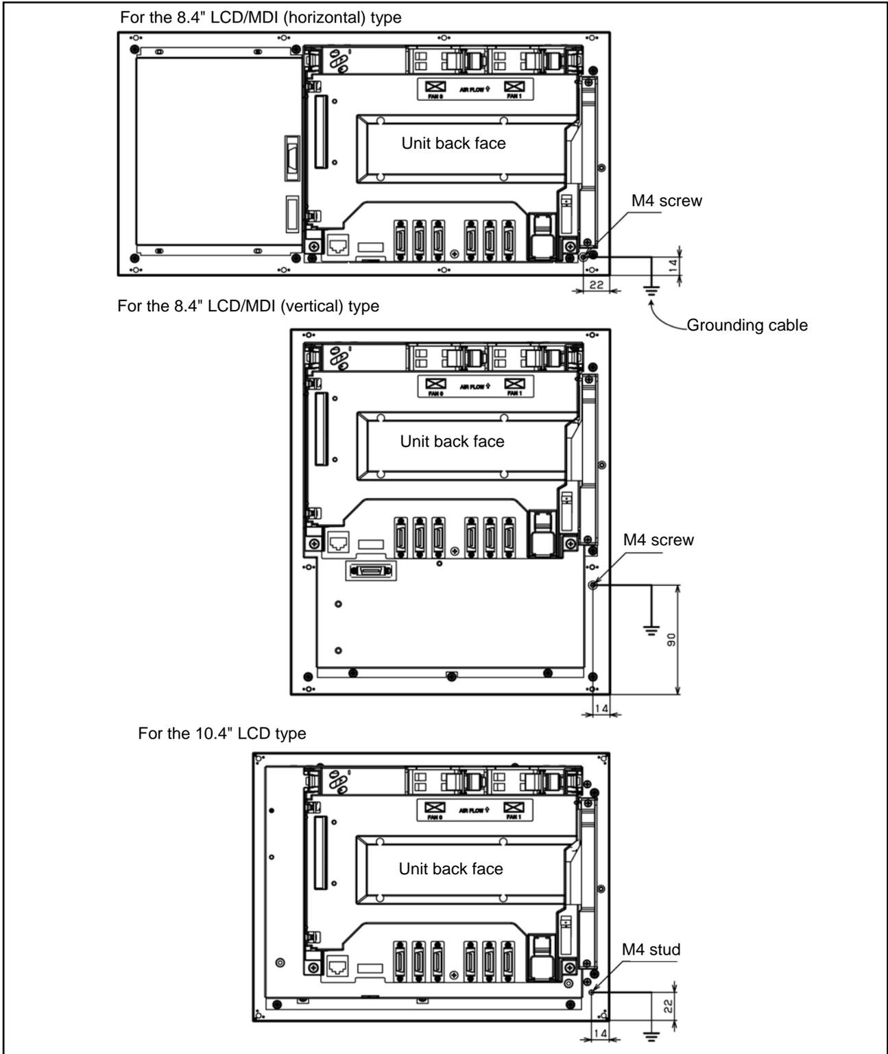
Connect the 0V line in the control unit to the ground plate of the cabinet via the protective ground terminal (shown in the above figure).
