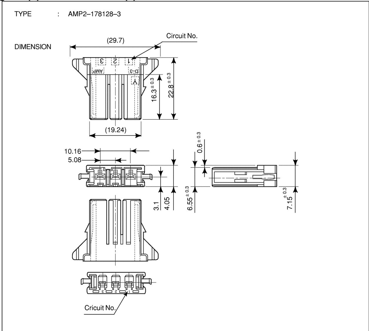
**Fig. C3 (c) AMP connector (3): For +24 V power supply**
