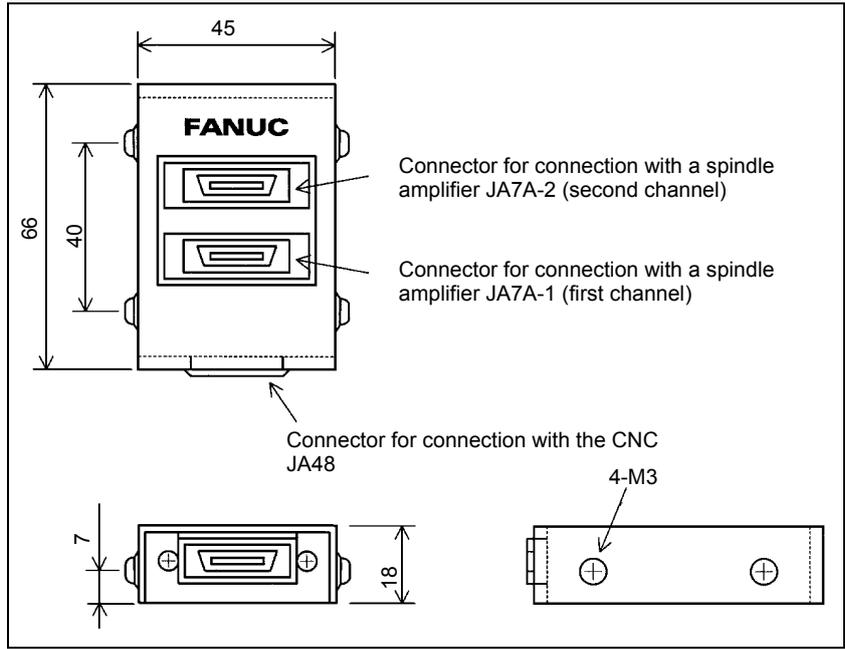
Conditions for installing the serial spindle connector panel
