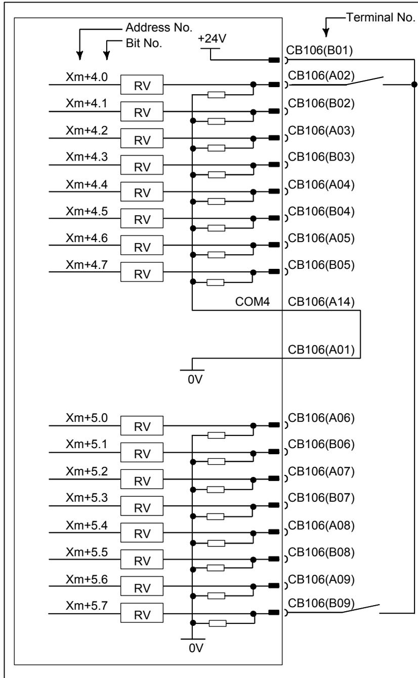
For address Xm+4, either a source or sink type (with a 0- or 24-V common voltage) can be selected. COM4 must be connected to either 24 or 0 V; never leave it open. From the viewpoint of safety standards, it is recommended that a sink type signal be used. The above diagram shows an example in which the signal is of sink type (with a 24-V common voltage).
