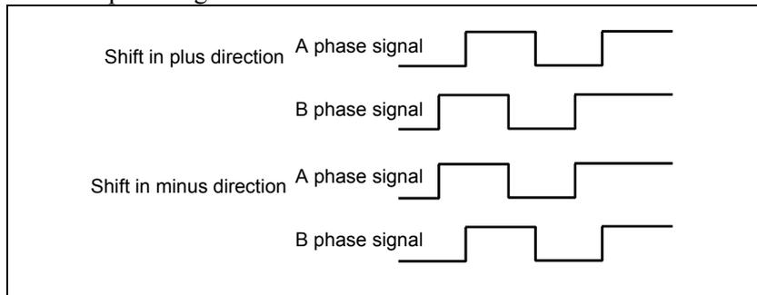
The differential input signals shown below are applied to the connectors. The time duration, TD, from point  $\alpha$  where the relative potential difference between A and \*A becomes 0.5 V or more, to point  $\beta$  where the relative potential difference between B and \*B becomes 0.5 V or less, must satisfy the condition indicated below. (This condition may restrict the maximum speed of movement.)
