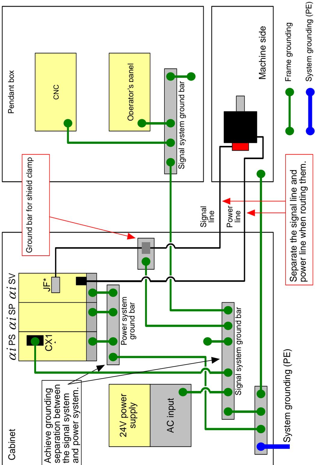
Fig. 3.5.1.2 (b) Schematic diagram for single-point grounding scheme
