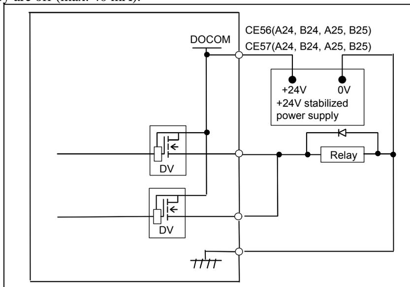
DO (output signal) alarm detection
