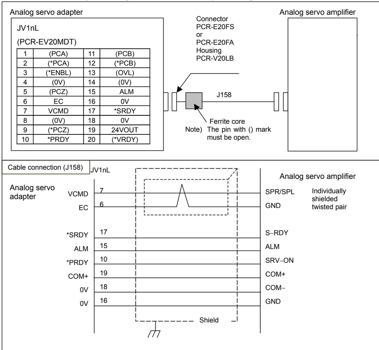
Maximum allowable cable length : 50m (cable length has limitation by voltage drop)
