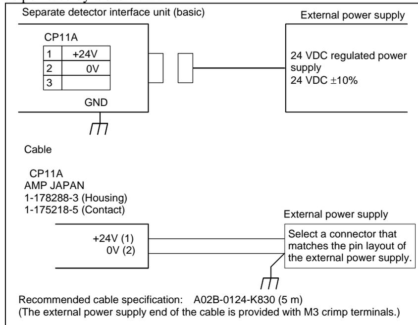
The 24 VDC input to CP11A can be output at CP11B for use in branching. The connection of CP11B is identical to that of CP11A. In this case, the power supplied to CP11A should be equal to the sum of the rating of the separate detector interface unit and that of the units after CP11B.
