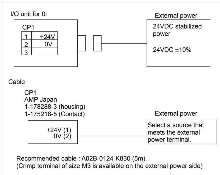
Part of the 24 VDC power input to CP1 can be taken out from CP2 by branching. CP2 should be connected as shown below. In this case, the rating of the external 24 VDC power supplied to CP1 must be the sum of the power consumed within the control unit and that supplied to external equipment via CP2. The maximum capacity of power that can be obtained from a branch is 1.0 A.
