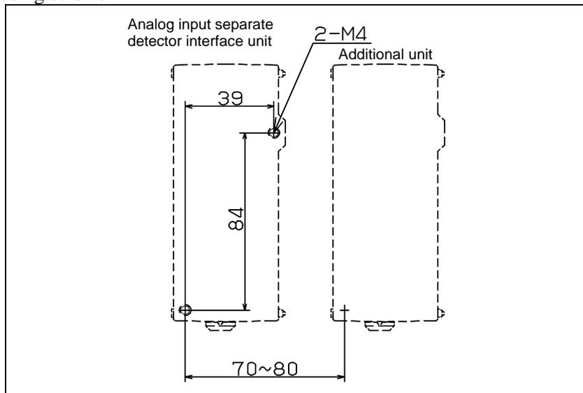
When using both an analog input separate detector interface unit and additional unit, install the units as shown above, with the mounting holes horizontally separated by 70 to 80 mm.
