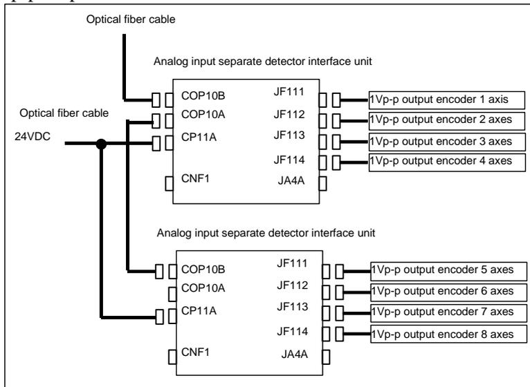
(3) Connecting 1-Vp-p output encoders to the 1st to 4th axes and digital output encoders to the 1st to 4th axes
