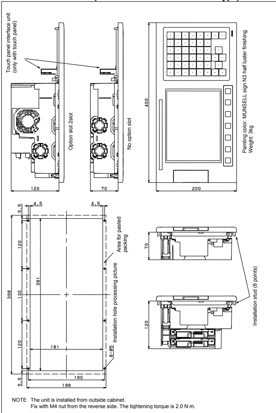
**Fig. U2 CNC control unit (8.4" color LCD/MDI vertical type)**
