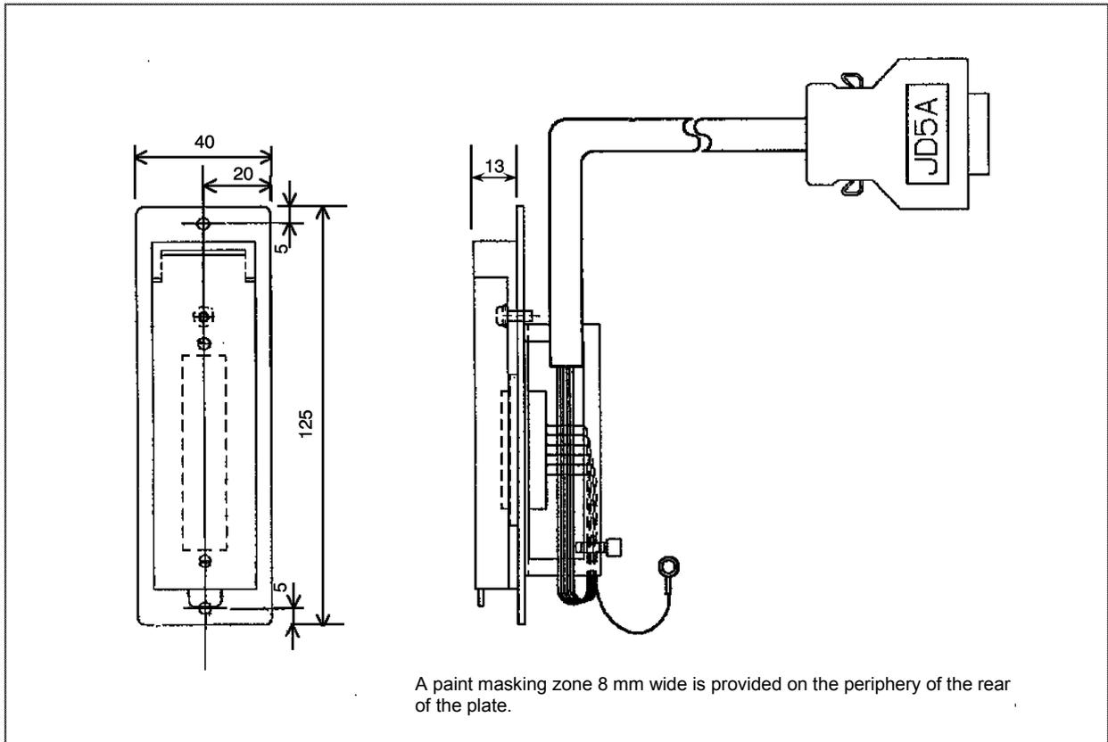
The panel cut dimensions of this punch panel are indicated below.
