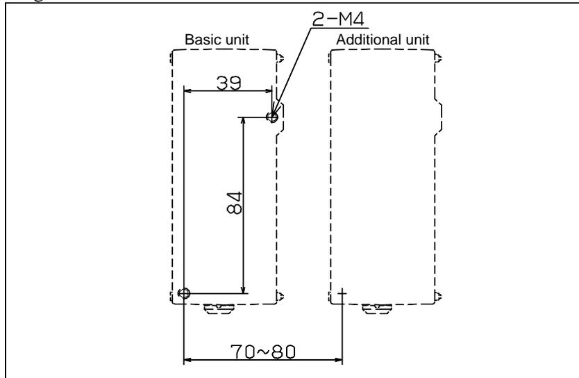
When using both a basic unit and additional unit, install the units as shown above, with the mounting holes horizontally separated by 70 to 80 mm.
