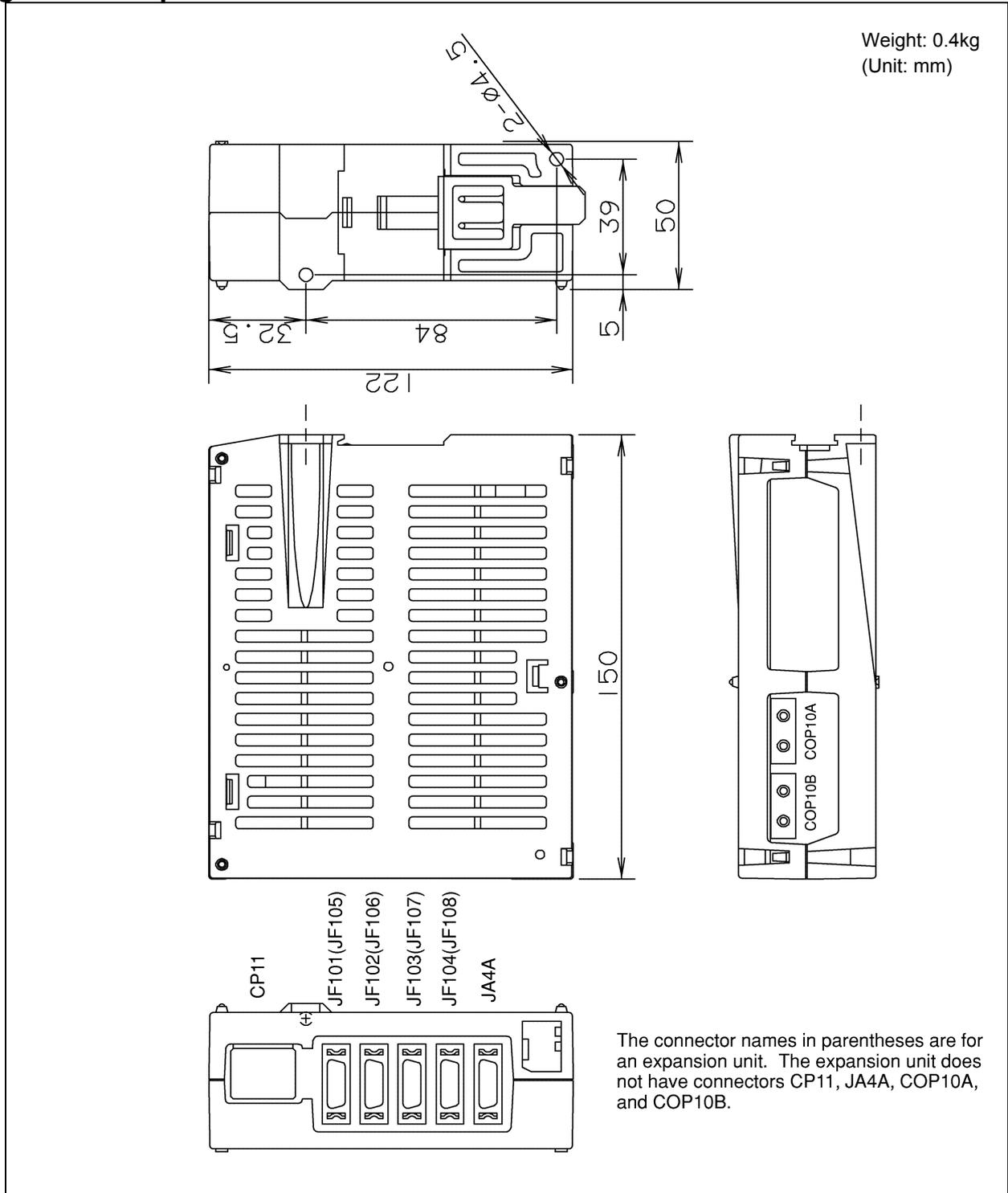
**Fig. U21 Battery case for separate detector interface unit (ABS)**
