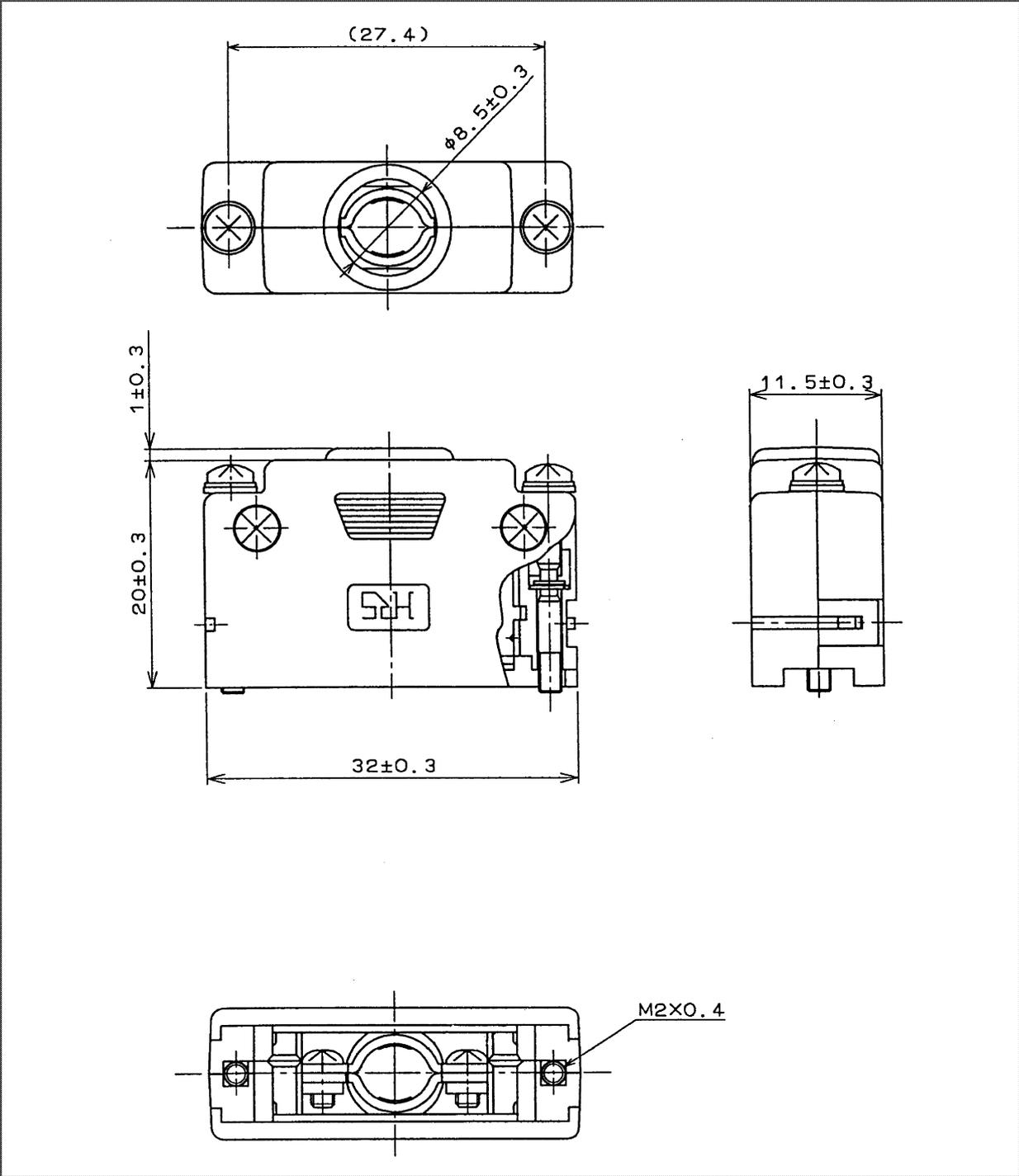
**Fig. C3 (a) AMP connector (1): On the servo side**
