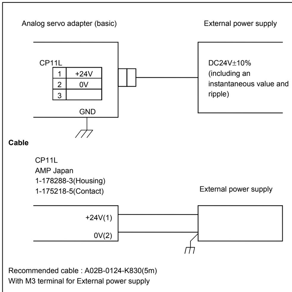
24VDC are supplied through the connector CP11L. The power can be supplied from CP11M to the next unit.
