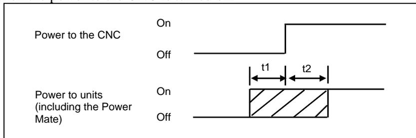
t1:200ms Means that the power to units (including the Power Mate) is turned on within 200 ms before the power to the CNC is turned on.
