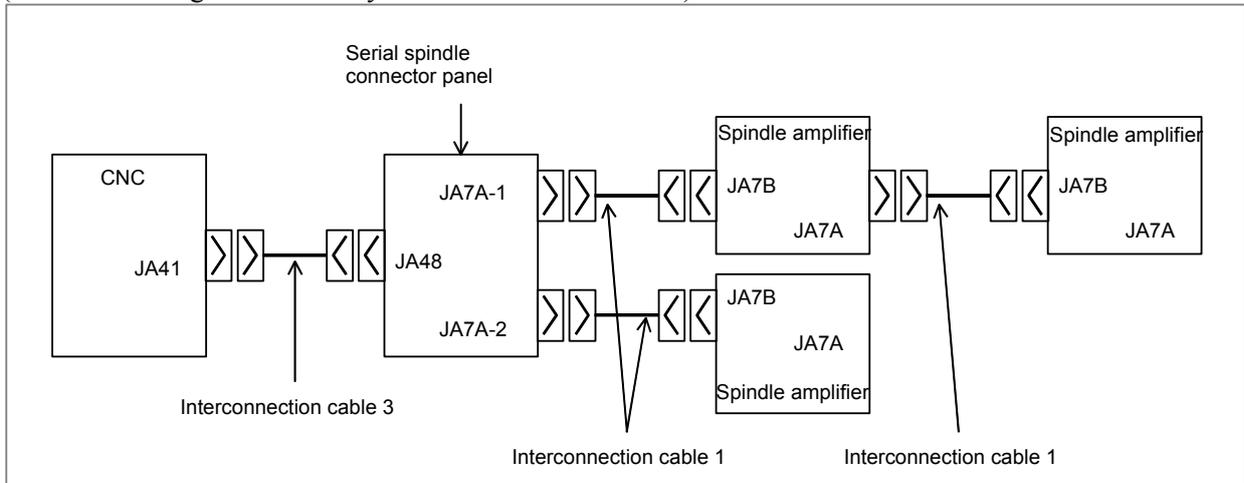
(Connection diagram when optical cables are used)
