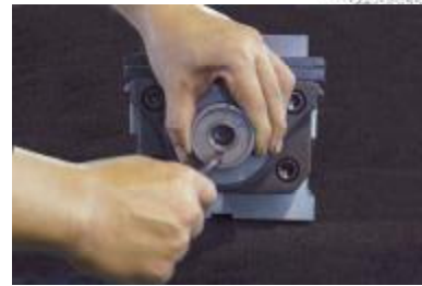
Now to adjust the clamping force
